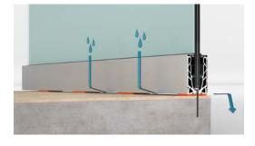
Perforated aluminium accessory to be placed at the base of the profile (no. 4 pieces per linear metre, at the fasteners to the substructure), in order to raise the whole system by 5 mm and allow water to drain off.
