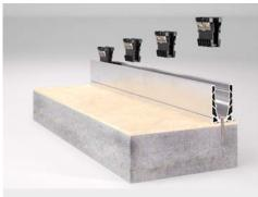
Lay the clamps inside the profile every 250 mm. Do not place the clamps over the fixing screws.
