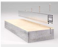
Perforate the slab with the drill, position the profile and the fixing screws.
