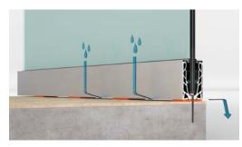
Perforated aluminium accessory to be placed at the base of the profile (no. 4 pieces per linear metre, at the fasteners to the substructure), in order to raise the whole system by 5 mm and allow water to drain off.
