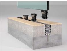
Lay the clamps inside the profile every 250 mm.
