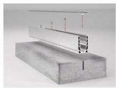
Perforate the slab with the drill, place the profile, fixing screws and temporary cover to prevent aggregates from soiling the profile during construction.
