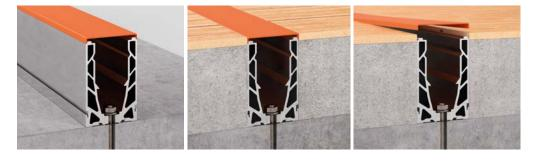
Provisional element applied as protection to the profile to avoid the entry of inerts during the completion phases of the construction site. It also provides the floor dimension reference.
